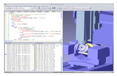
$Integrated \ APT/CL, \ G\text{-}code \ and \ machine \ view \ provide \ the \ complete \ picture \ for \ CNC \ post \ development.$
