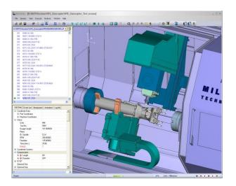
IMSverify 2011 provides machine simulation with collision detection for all types of machine configurations – milling, turning and mill/turn.
