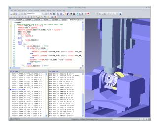
Integrated APT/CL, G-code and machine view provide the complete picture for CNC post development.
